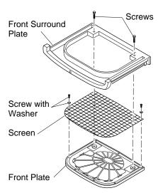
Figure 14 - Removing Screen from Front Assembly
